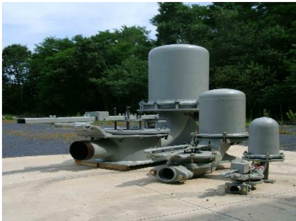
Figure.15 80HDU ram pumps & multiple rams with common delivery pipe
