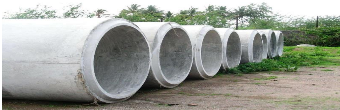
Figure.28 R.C.C pipe of 2.2 m in diameter
