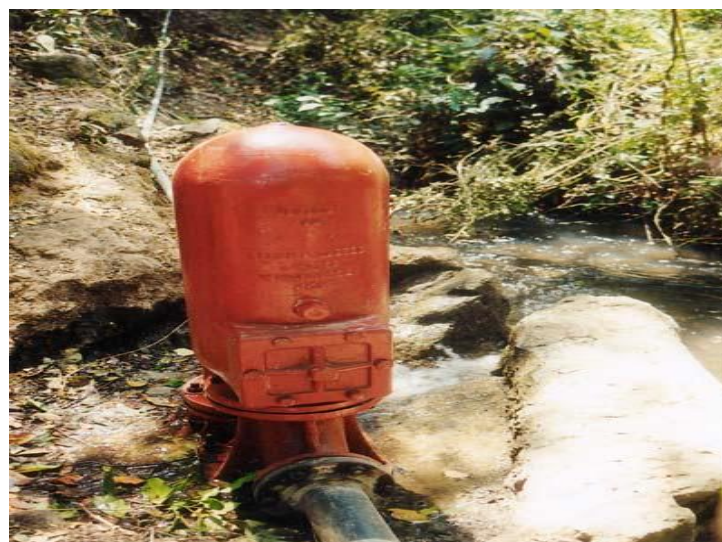
Figure.9 The hydraulic ram pump (Old model)
